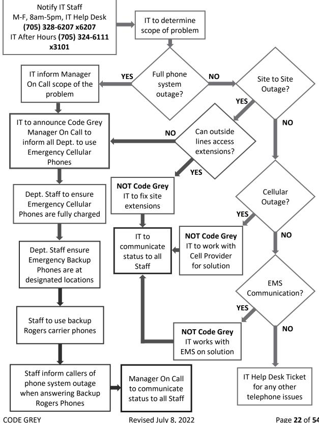
Appendix 3 – Telephone System Failure - Algorithm
